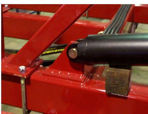
Fig 1. When charging the circuit, prop up cylinder with block of wood. Be sure the rod can extend freely without striking anything.
